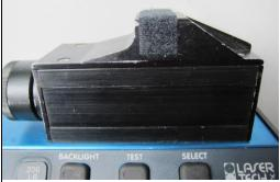
Install face plate urethane foam pad to the Lidar gun aluminum face clean the face plate and carefully center the adhesive pad to the gun. With the padding on the gun rather than the holster, you can easily wash the holster periodically and the padding is less likely to deteriorate due to environmental influences. Replacement urethane foam pads and Velcro are available from FMS Accessories.
